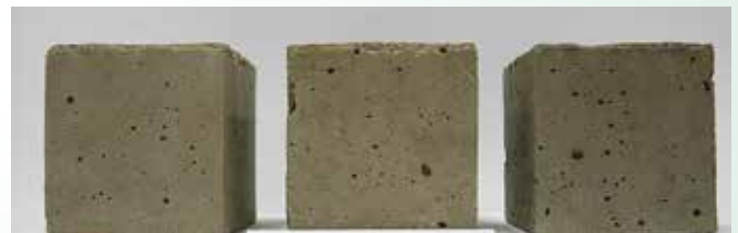
Developed sulphur concrete exposed to water (Undamaged)
