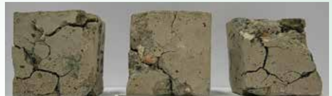
Conventional sulphur concrete exposed to water (Damaged)
