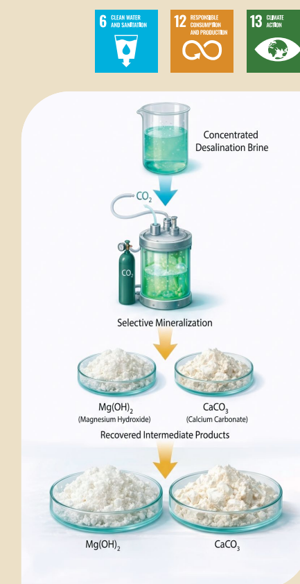
Recovered minerals from desalination brine using CO 2 -assisted selective mineralization processes.
