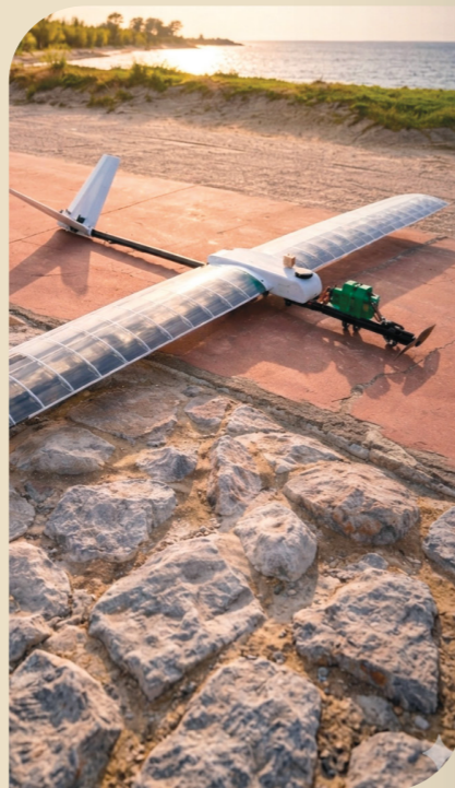
Solar-battery hybrid UAV enabling low-emission infrastructure inspection with onboard AI and extended endurance.
