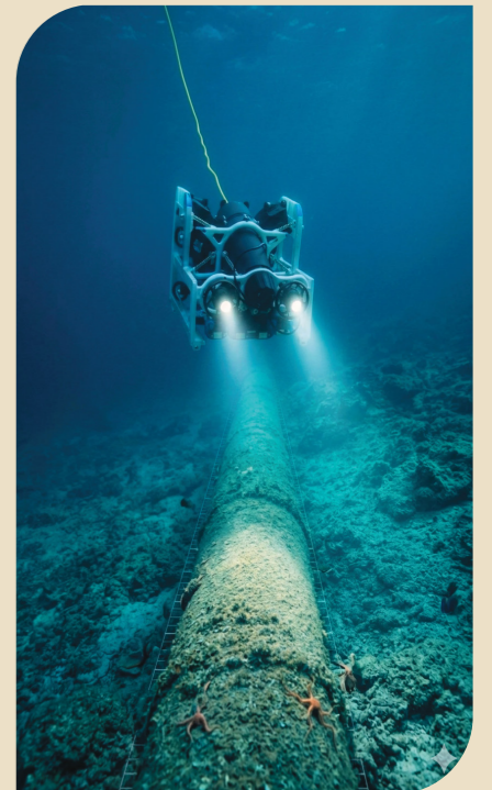
Marjan-R1 remotely operated vehicle (ROV) performing subsea inspection at TRL 6.
