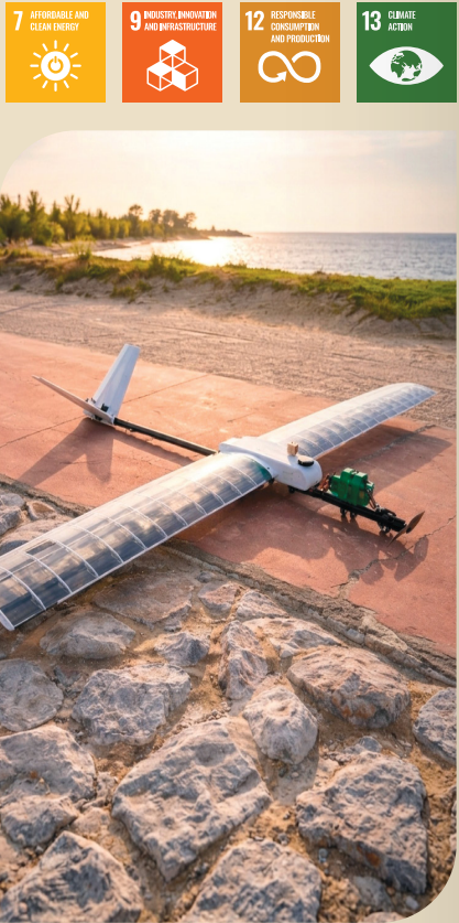
Solar-battery hybrid UAV enabling low-emission infrastructure inspection with onboard AI and extended endurance.
