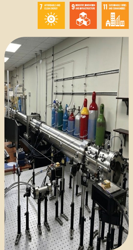
Advanced shock-tube diagnostics platform generating high-precision data for lithium-ion battery safety modeling.
