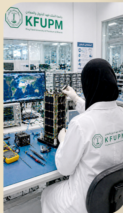
CubeSat assembly and integration facility supporting hyperspectral Earth observation and in-orbit validation.
