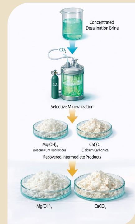
Recovered minerals from desalination brine using CO 2 -assisted selective mineralization processes.
